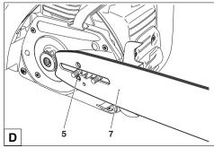
Put on the guide bar (7). Make sure that the pin (5) of the chain tensioner engages in the hole in the guide bar.
