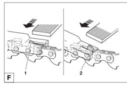
After having sharpened the chain, the height of the depth limiter must be checked by means of a chain gauge. See "Accessories" for the order number.
