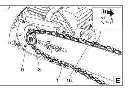
Pull the chain (9) around the sprocket nose (12) of the guide bar in the direction of the arrow.
