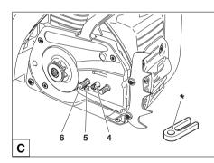
Remove the plastic transport cover (\*) and dispose of properly.
