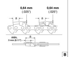
The sharpening angle (a) must be identical for all cutters!
