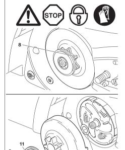
Check the sprocket before mounting a new chain.
